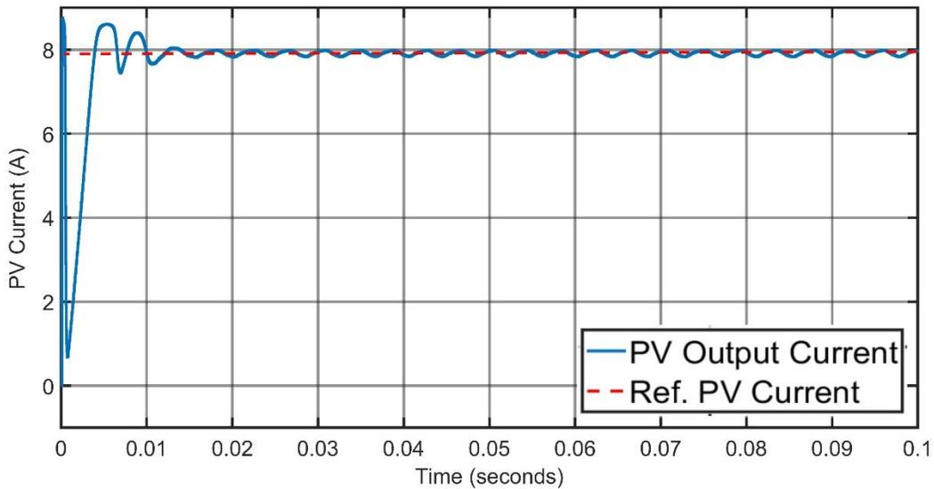
**Figure 12** Output current from the PV system under constant atmospheric conditions.
