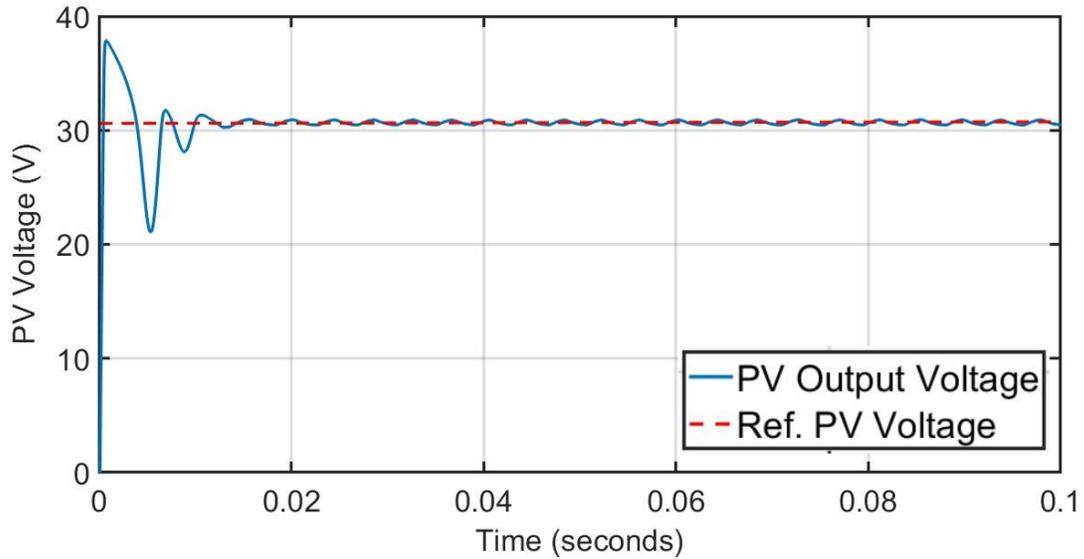
**Figure 11** Output voltage from the PV system under constant atmospheric conditions.
