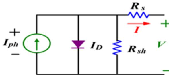
**Figure 2** PV cell equivalent circuit.
