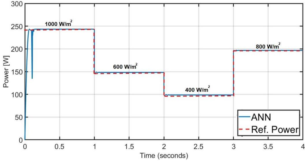
**Figure 13** PV module output power at varying irradiance levels and constant temperature.
