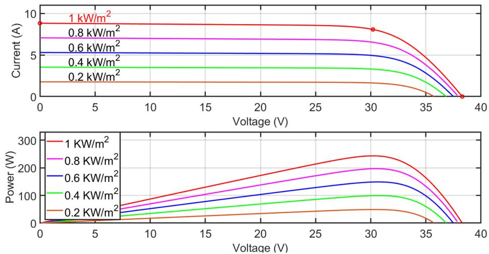
Figure 8 PV module characteristics at constant temperature and varying irradiance levels.
