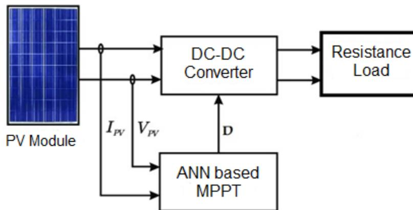
**Figure 1** Schematic diagram of the proposed system.
