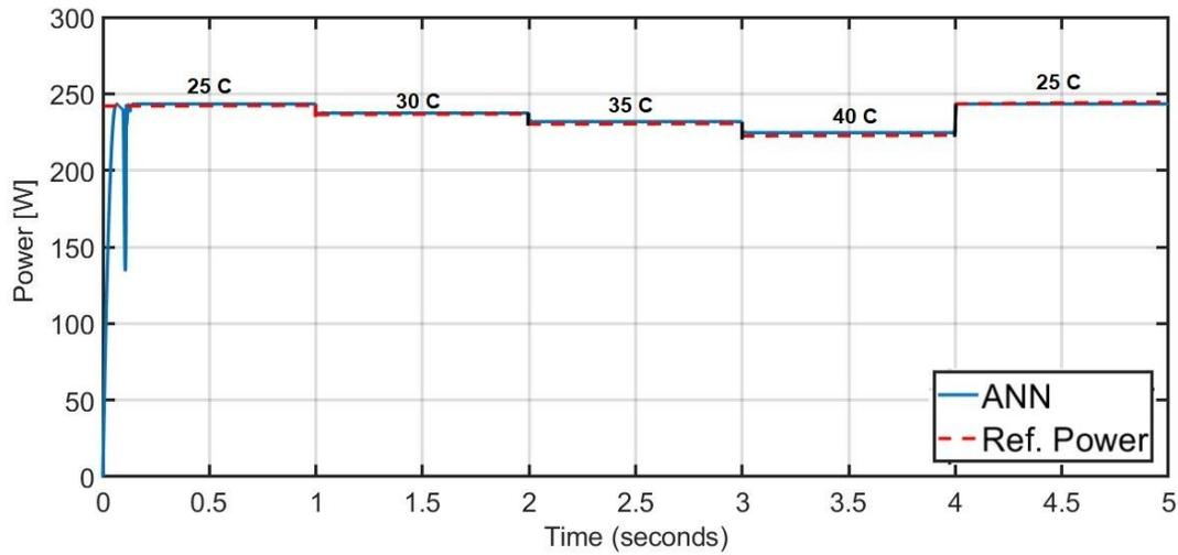
**Figure 14** PV module output power at varying temperature levels and constant irradiation.
