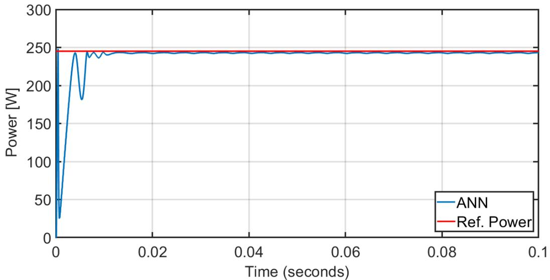
**Figure 10** Output power from the PV system under constant atmospheric conditions.
