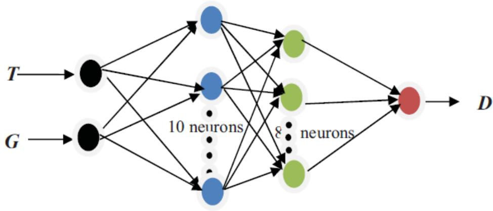
**Figure 5** Proposed feedforward NN structure.
