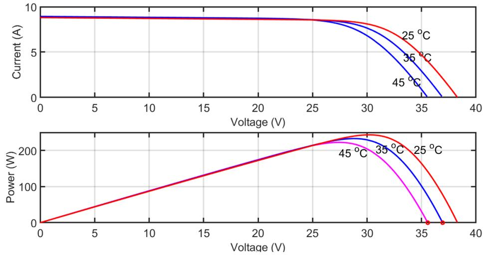
**Figure 9** PV module characteristics at varying temperatures and constant irradiance levels
