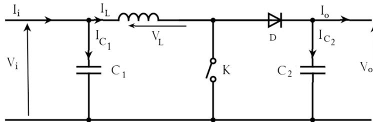
**Figure 3** Circuit diagram of the converter.
